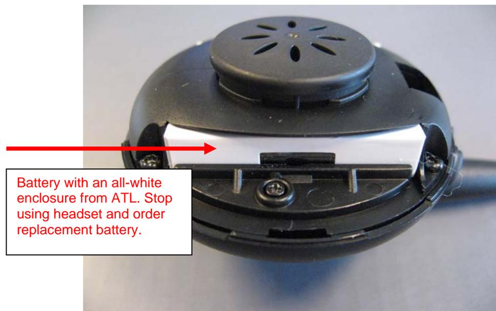
**Battery with white plastic enclosure AND Made by Synergy sticker is *outside scope of replacement* program**
