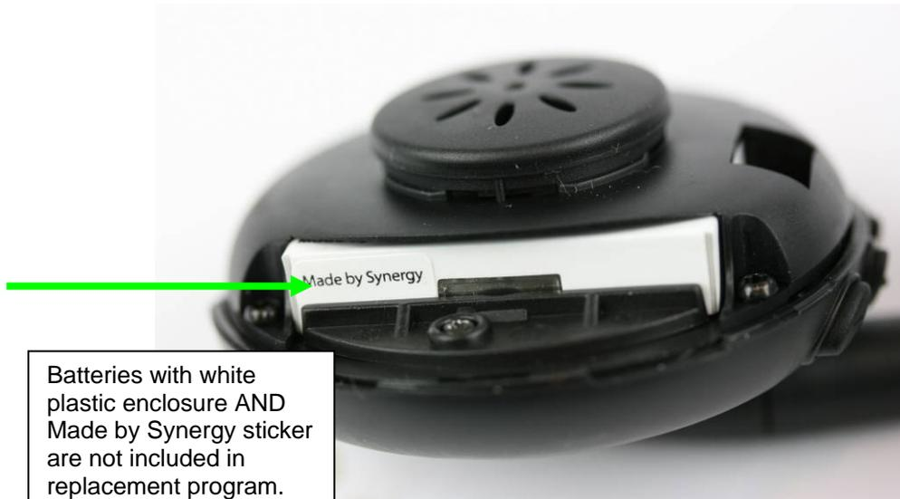
Batteries with white plastic enclosure AND Made by Synergy sticker are not included in replacement program. Continue use of headset.
